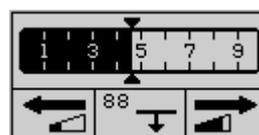
Now the sensitivity of the receiver can be decreased by one percent by pressing the 1 button, or increased by one percent by pressing the 3 button. This process can be accelerated by holding down the respective button.
