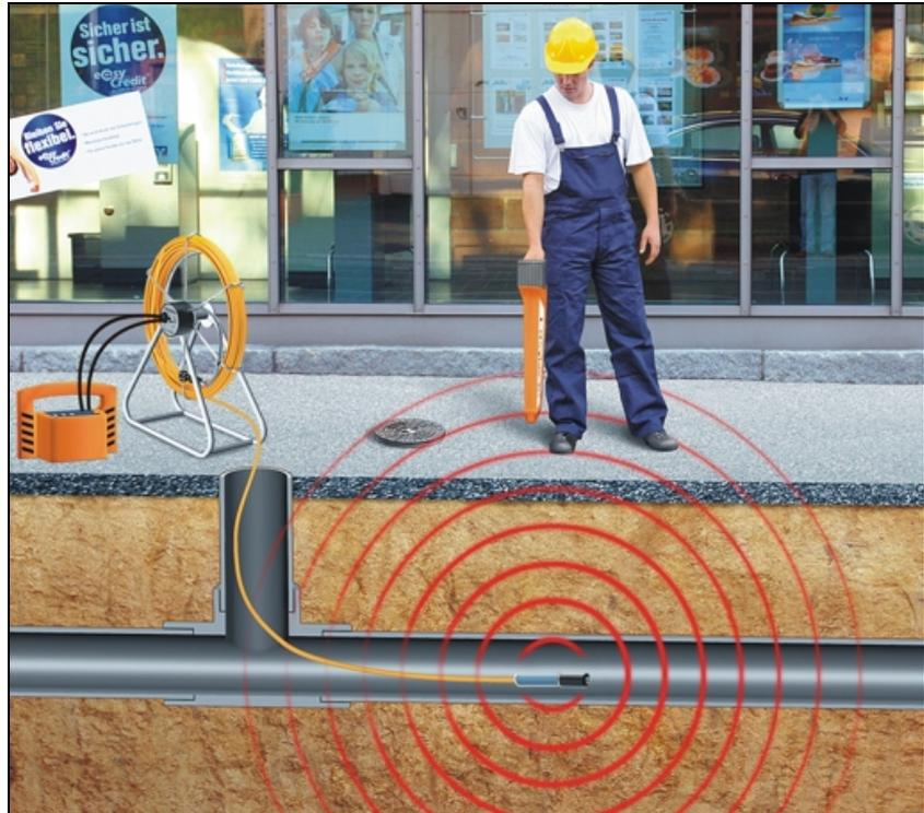
Alternatively, any other active probe (e.g. a camera probe) with adequate transmitting frequency (see Technical Data) can be located using the receiver. For a detailed description, please refer to the manual of the respective product.
