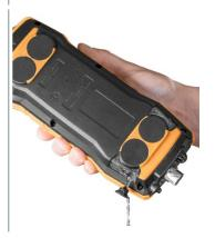
Wipe off any drops still on the condensate outlet with a cloth and close the condensate outlet.
